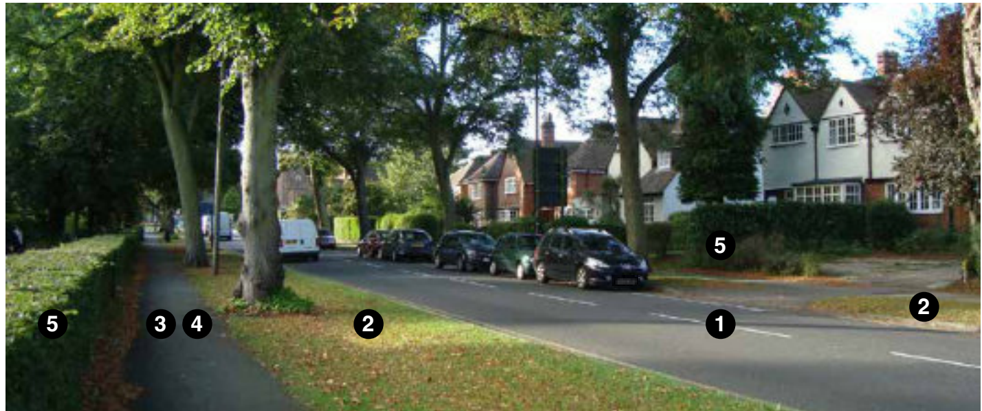
Figure 33: Primary road framed by wide tree verges in a residential neighbourhood. It is recommended that cycle provisions are separated from moving traffic and that parking bays, where required, are inset into the verges to avoid impeding the movement of pedestrians and vehicles.
