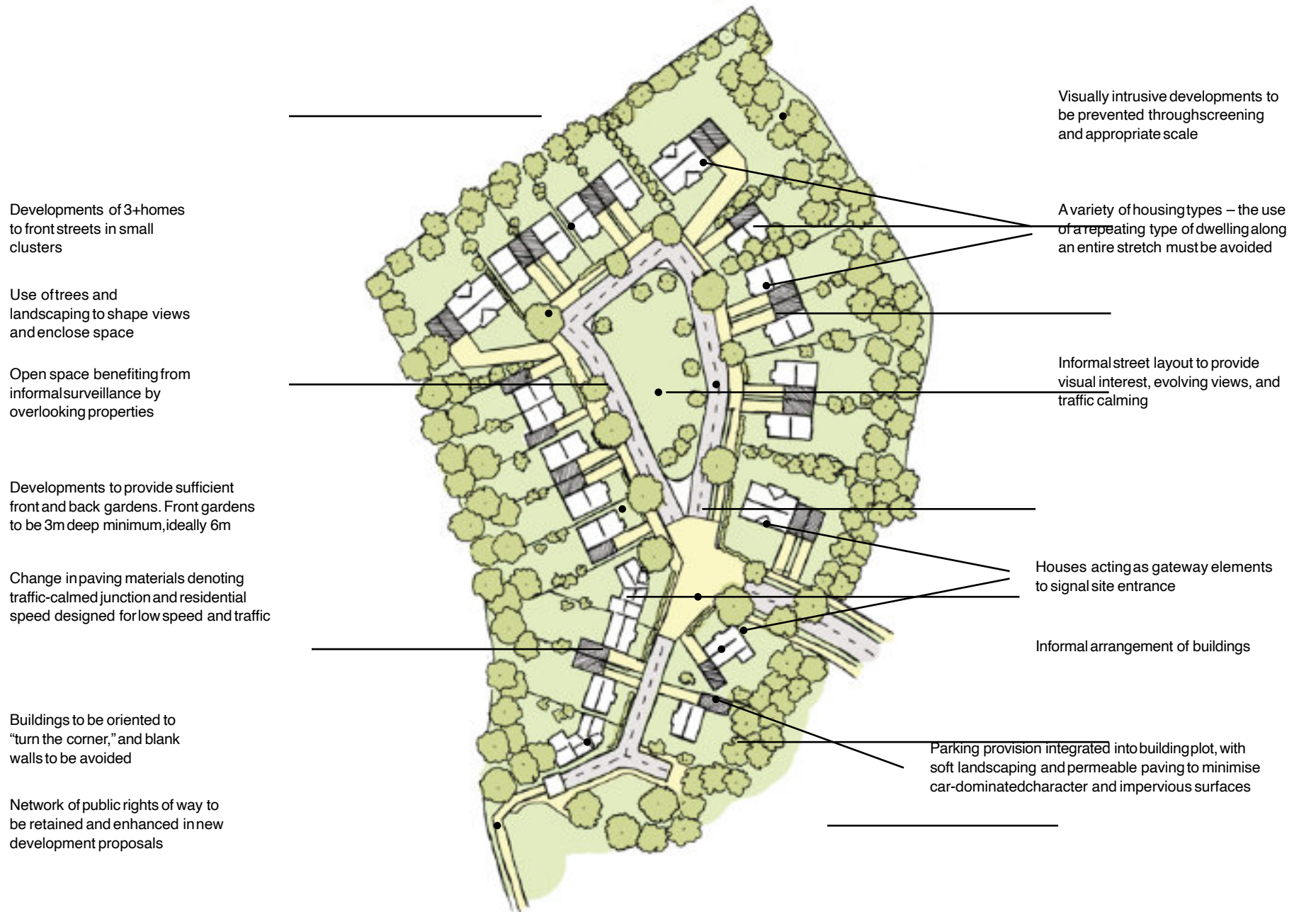
Figure 19: Illustrative plan for a small development highlighting many of the elements of the Sarratt code where they relate to the pattern and layout of buildings.
